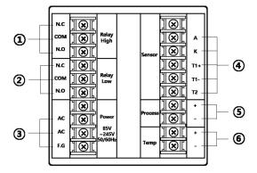
① Relay High: HIGH Alarm Output Terminal
